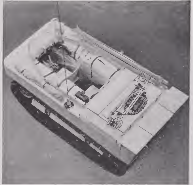
FIGURE 22. Top view of final pilot model of T-15 Weasel, showing accommodations for driver and one passenger.
